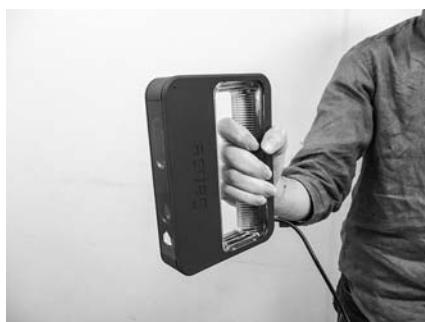
図10 SENSE 3D Scanner
