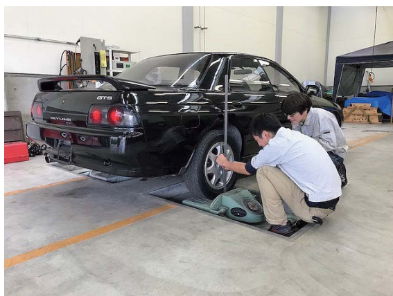
Fig. 4 Measurement of suspension stroke in wheel edge
