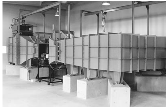
Fig. 3 Goettingen type scale model wind tunnel used in car design
