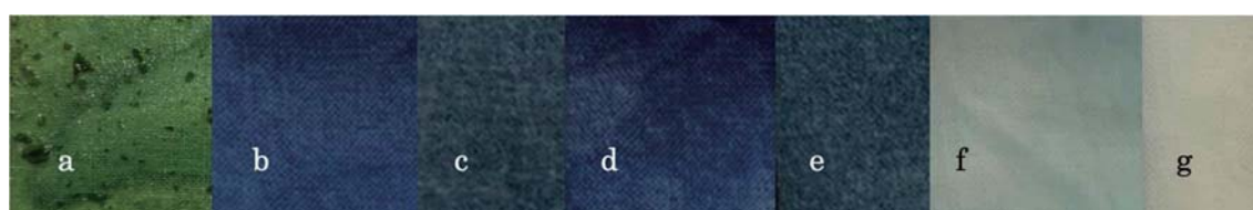
Fig. 9 Indigo dyeing of cotton; (a) before oxidation, (b) rinsed in water, (c) rinsed in water after protein coating, (d) oxidated, (e) oxidated after protein coating, (f) added Sodium hydrosulfite, (g) added Sodium hydrate.
