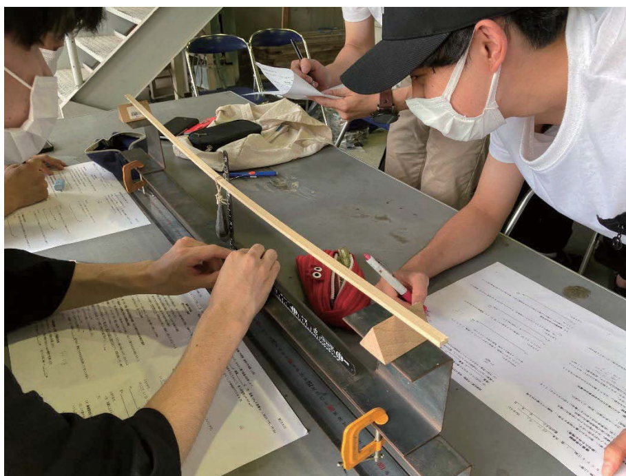
Photo 2 Deflection measurement of the test
