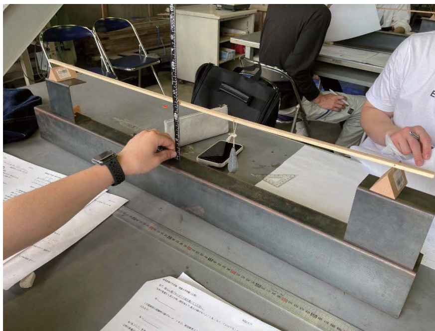
Photo 4 Test of the superposition principle
