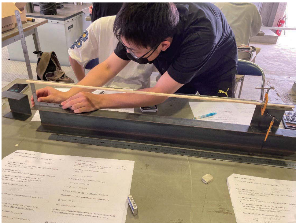
Photo 3 Measurement of a cantilever beam
