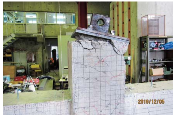
Photo 4 Failure at column top of No. 2
