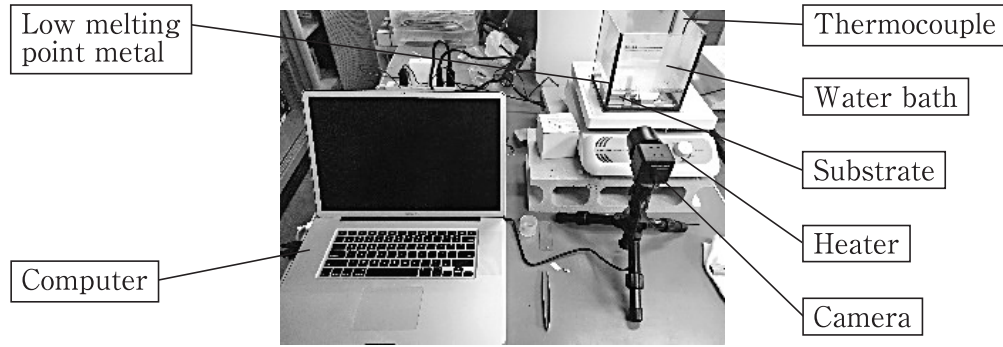
Fig.2 Experimental setup of wettability measurements in hot water
