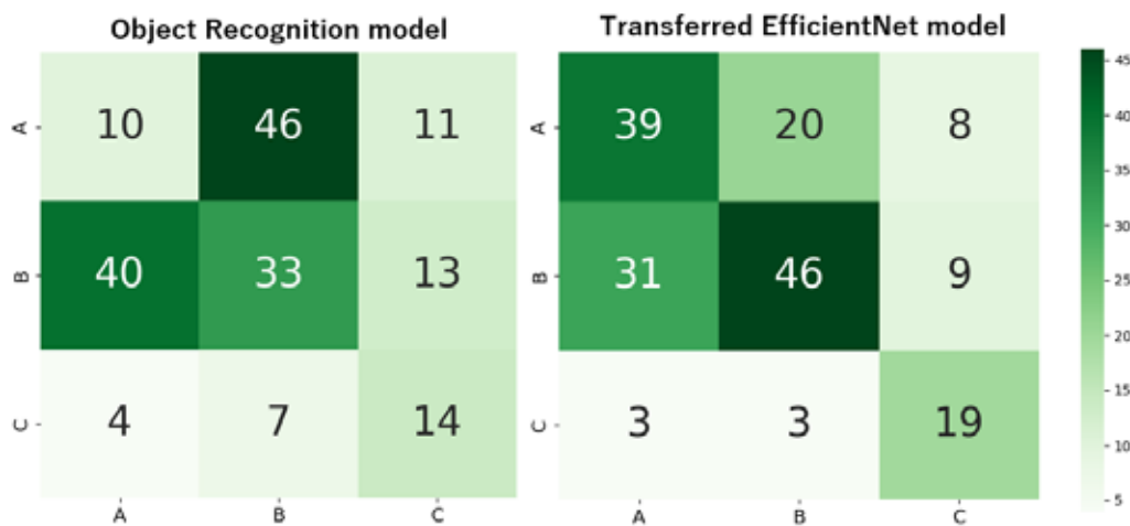
Fig. 7 Comparison of confusion matrix for 3-class classification prediction using object recognition model and transferred EfficientNet
