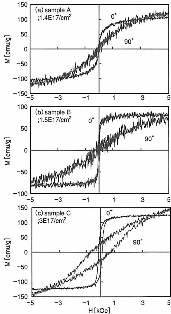
Fig. 3; Magnetization curves taken from iron implanted a- $\text{SiO}_2$ , sample A with a dose of  $(1.0+0.4) \times 10^{17}$  ions/cm<sup>2</sup>, sample B with  $1.5 \times 10^{17}$  ions/cm<sup>2</sup>, and sample C with  $3.0 \times 10^{17}$  ions/cm<sup>2</sup>
