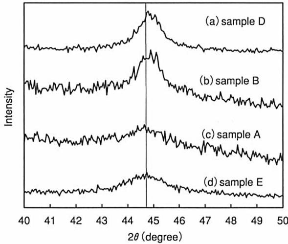
Fig. 2; GXR patterns from the implanted layers of the sample A (Fe/ $\text{SiO}_2$ ), sample B (Fe/ $\text{SiO}_2$ ), sample D (Fe/ $\text{SiO}_2$ ), and sample E (Fe/ $\text{Al}_2\text{O}_3$ ). The vertical line indicates the (110) diffraction angle of bulk iron.
