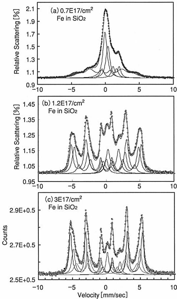
Fig. 4; CEM spectra of the Fe/SiO<sub>2</sub> granules from iron implanted a-SiO<sub>2</sub>; (a) with a dose of  $0.7 \times 10^{17}$  ions/cm<sup>2</sup>, (b) with  $1.2 \times 10^{17}$  ions/cm<sup>2</sup> and (c) with  $3.0 \times 10^{17}$  ions/cm<sup>2</sup> (sample C)
