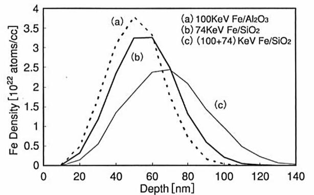
Fig. 1; Fe ions distribution calculated from TRIM code for the sample E (Fe/ $\text{Al}_2\text{O}_3$ ), sample B (Fe/ $\text{SiO}_2$ ), and sample A (Fe/ $\text{SiO}_2$ )
