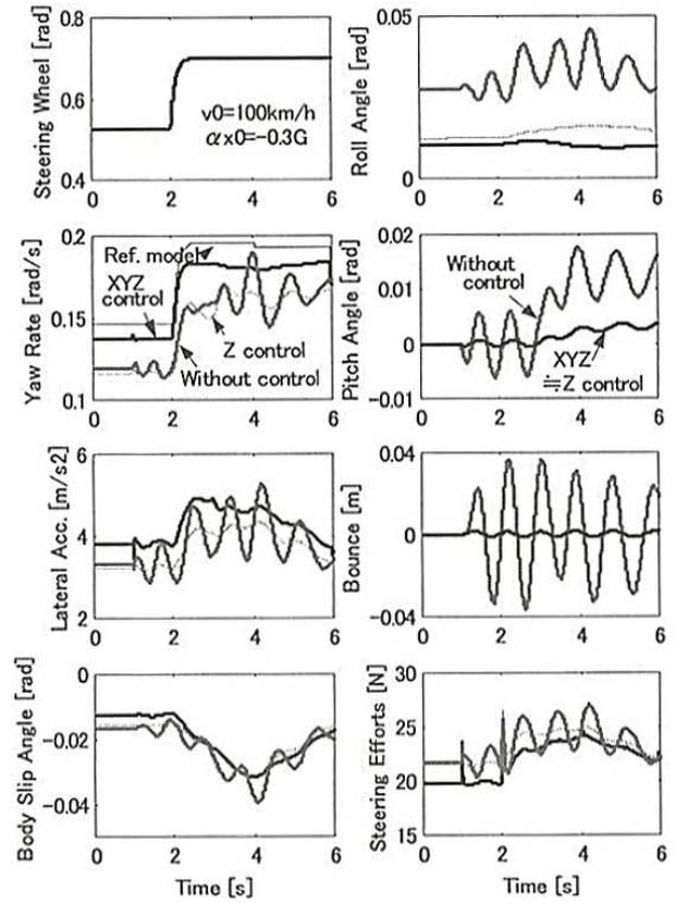
Fig. 3 Vehicle motion on the undulated road
