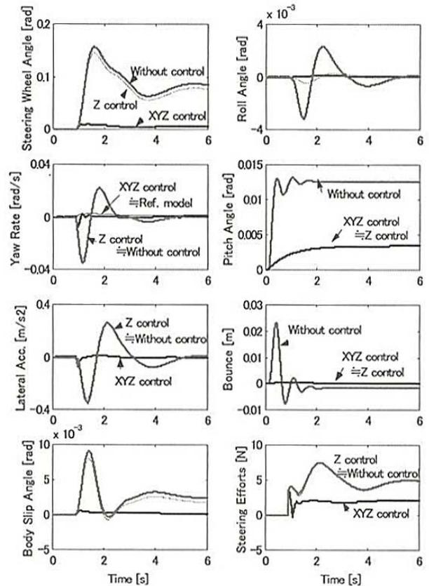
Fig. 8 Vehicle motion on the sprit  $\mu$  road
