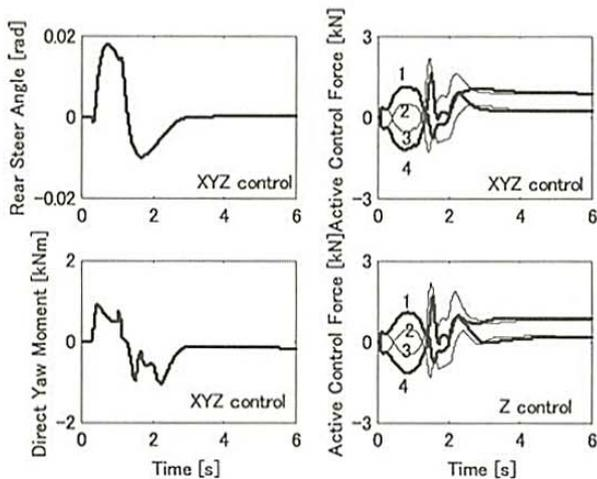
Fig. 6 Control input on the rut road
