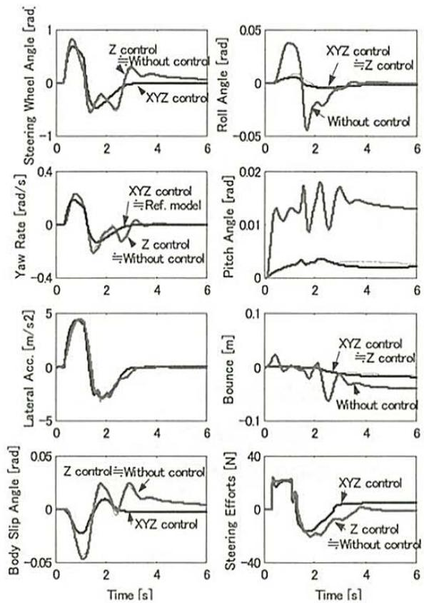
Fig. 5 Vehicle motion on the rut road
