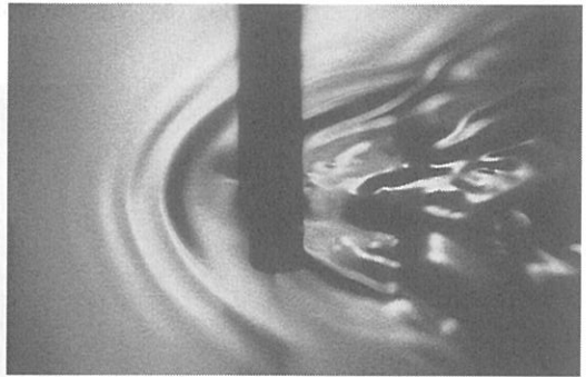
(e) d=1.1\text{cm} , U=28\text{cm/s} ( R=2.3 \times 10^3 , F=0.84 , W=21.0 )
