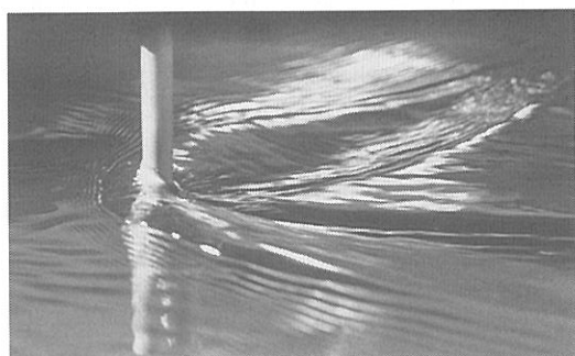
(a) d=1\text{cm} , U=50\text{cm/s} ( R=3.9 \times 10^3 , F=1.60 , W=34 )
