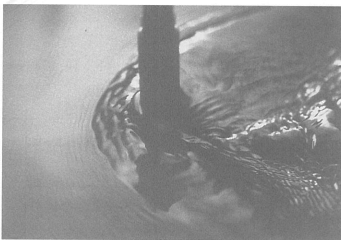
(a) d=1.5\text{cm} , U=55\text{cm/s} ( R=9.4\times 10^3 , F=1.43 , W=64.8 )
